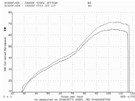
This graph shows a typical gain with a Dynojet jet kit.
